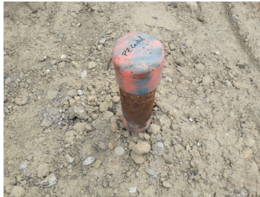
Pz central (ex Drain Central)
